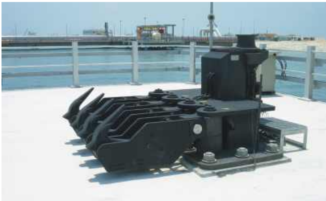
Figure 5. Quad hook with hydraulic release.
