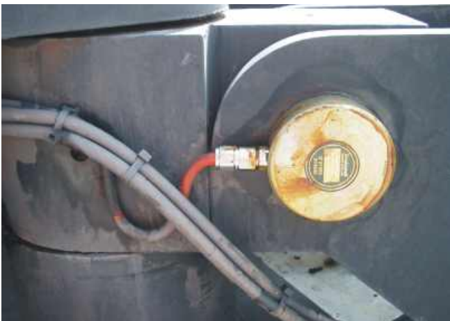
Figure 3. Load measuring pin installed into quick release mooring hook.
