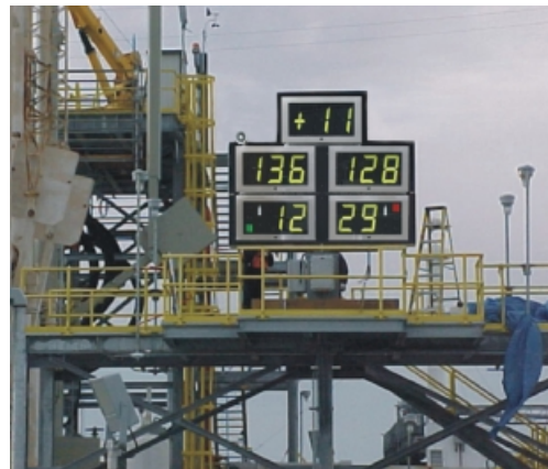
The Berthmanager display unit's modular design enables it to be easily upgraded and serviced on site
