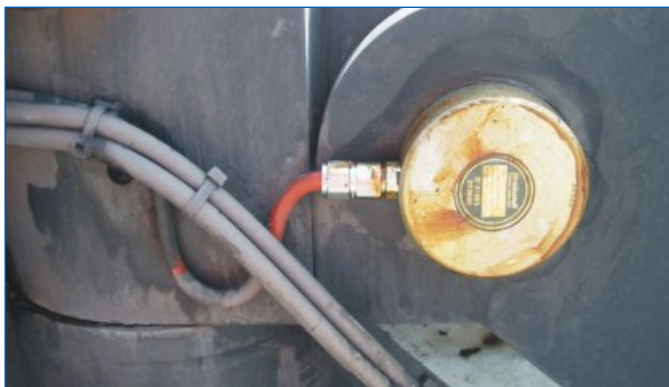
Figure 1. Load Measuring Pin installed into quick release mooring hook.
